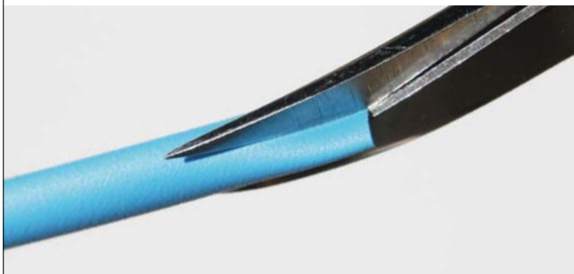
1 Cut the damaged tubing
