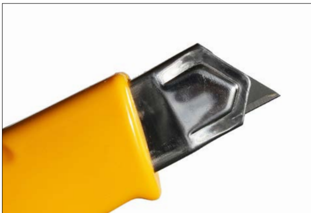
Box Cutter or Razor Blade— for trimming shrink tubing or plastic parts
