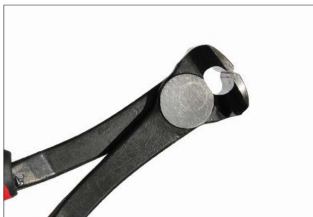
Front cutter—for cutting thicker wire or temple ends
