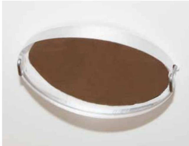
5. Fix the +6.0 D lens by means of a half frame from INSIDE the paper ring.
