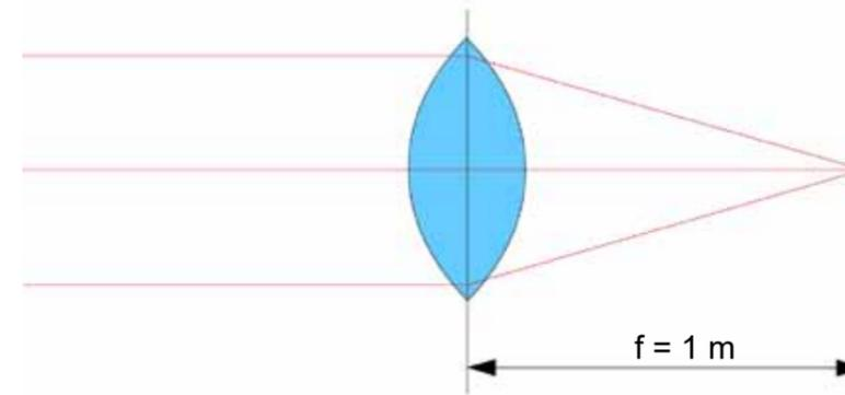
This lens has a focal length of  $f = 1 \text{ m}$
