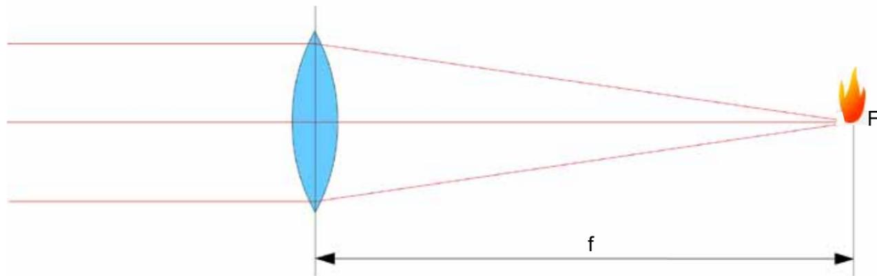
The **focal length f** is the distance between the centre of the lens and the focal point F.
