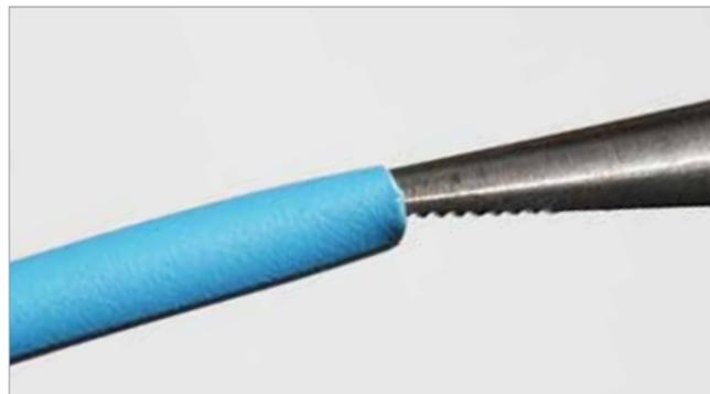
4. Tuck the cut end into the tube
