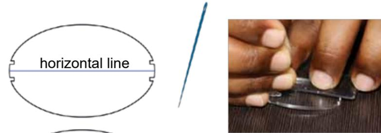
Now scratch a mark 21 mm from the left side into the lens.
