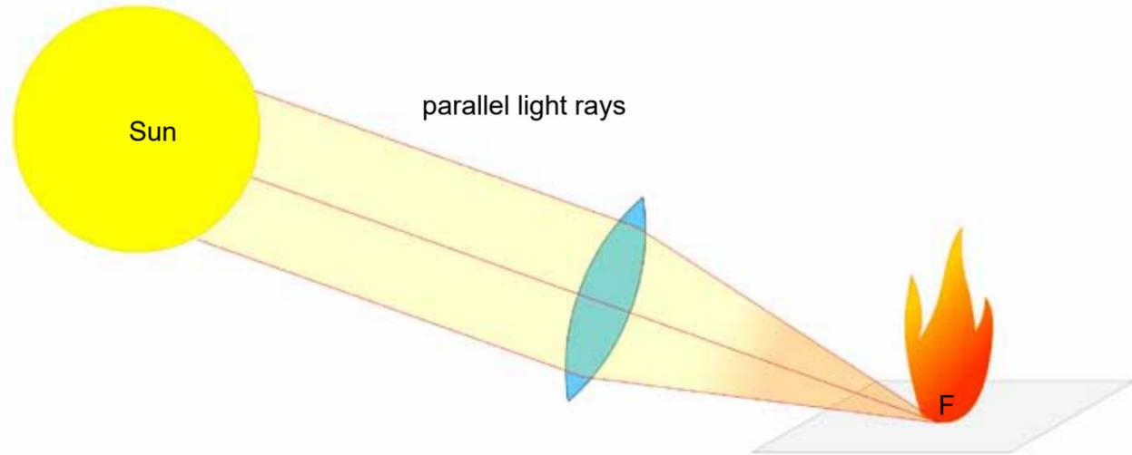
If parallel light rays pass through a positive lens, they get focused in one point, the **focal point F** (or focus). At this point a piece of paper starts to burn.
