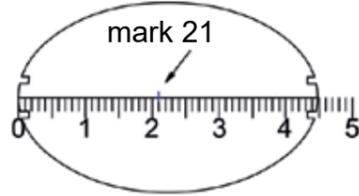
Now scratch a second mark 24 mm from the left side into the lens.
